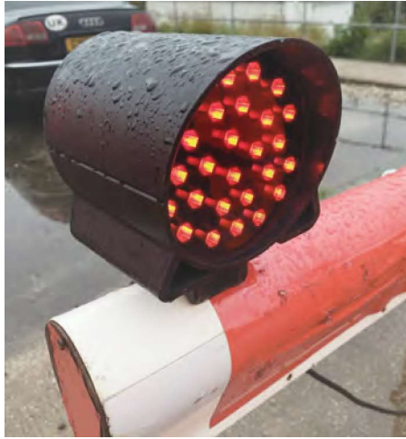
Retrofitted boom lighting is another approach
