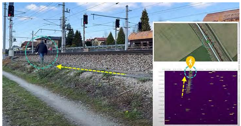
Figure 6 – Video image from security application demonstration. Inset bottom shows the recorded vibration created by the footsteps, and the inset top shows geolocated location.
